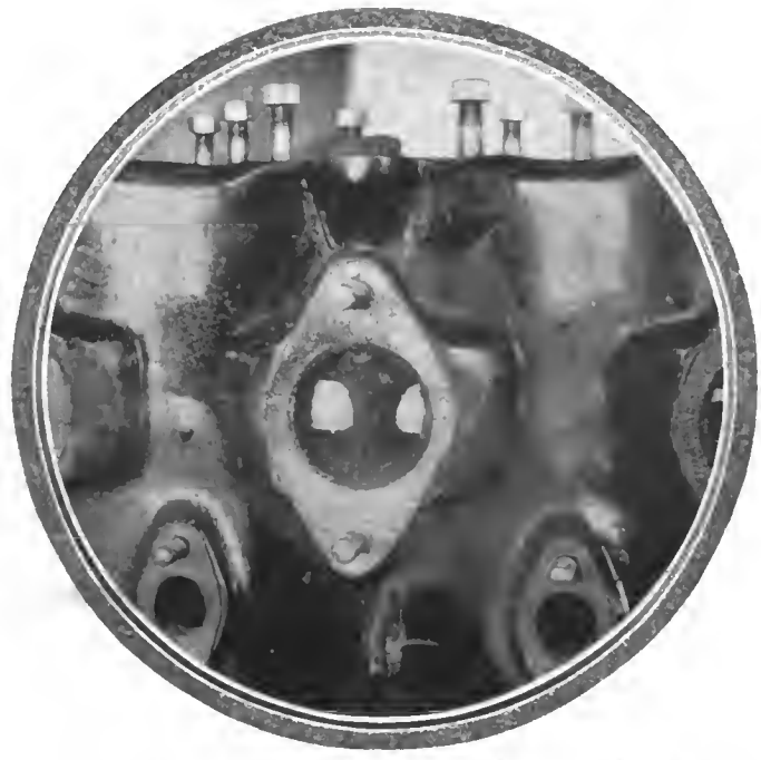
Fig. 18—Exhaust side of Stoddard-Dayton-Knight motor, showing central web in the passage-way forming a support for connecting piece in sleeve
